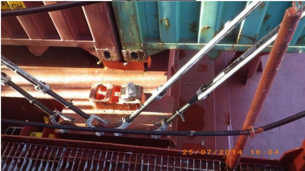
Picture of other deficiency: Numerous CO2 bottles securing arrangements loose
