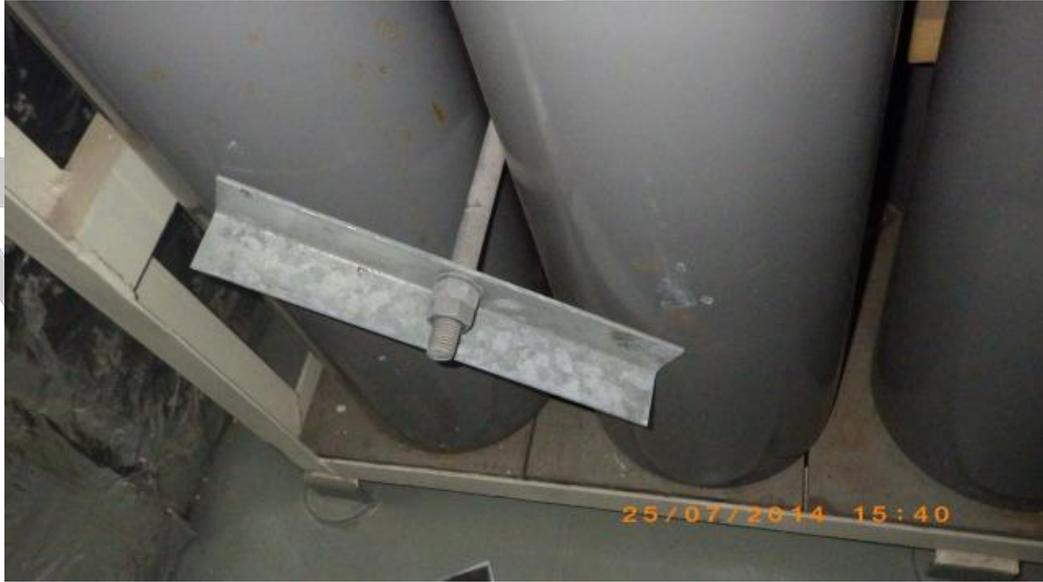
Picture of other deficiency: Both port and starboard lifeboats release system: stop lever B not re-set
