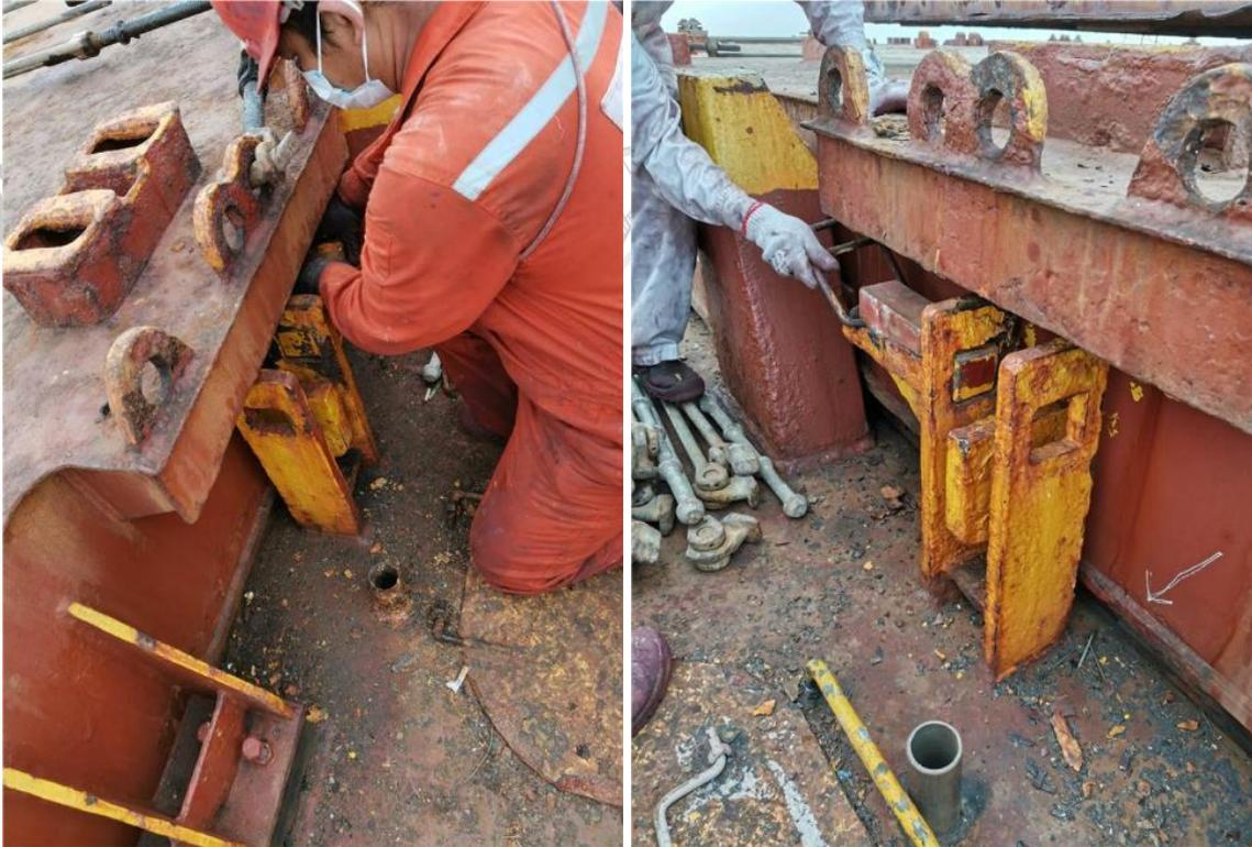
Pictures of detainable deficiency: Both the fire hydrants of spray fire protect for No.2 cargo hold are unable to connect with the fire hose due to serious corrosion
