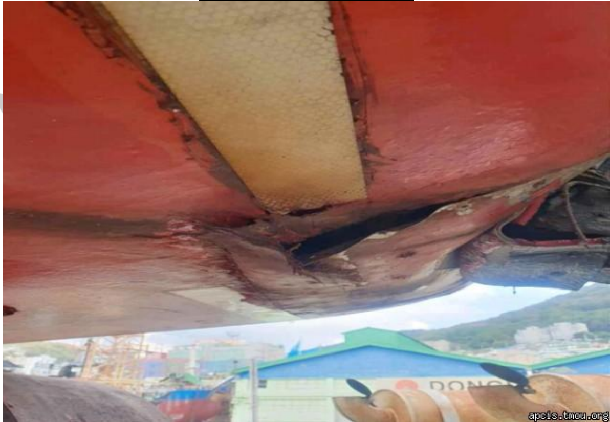
Picture of other detainable deficiency: Rescue boat on boat-deck starboard side found hole on bottom.
