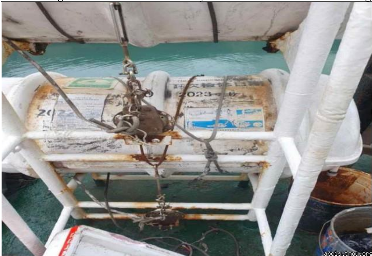
Picture of other detainable deficiency: Inflatable liferafts not working properly - interval of serviced date exceed 12 months (last service date: 06-2023) - fail to launching inflatable liferaft because hydrostatic release unit not working.
