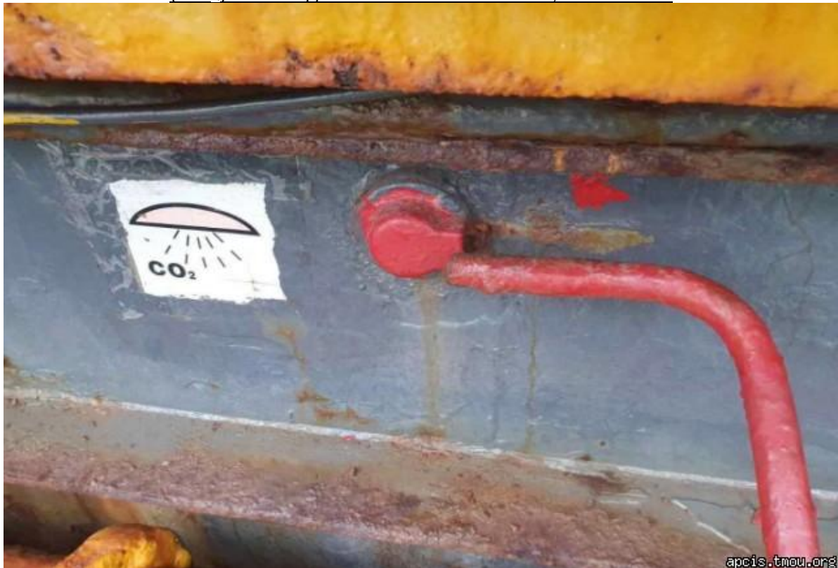
Picture of other detainable deficiency: Pipe of fixed fire-extinguishing system (CO 2 ) for cargo hold cut and heavily corroded.
