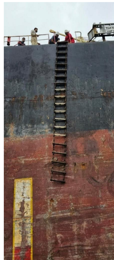
Figure 4. Incorrect ladder used, no spreaders, and combination arrangement not provided for safe embarkation to the vessel despite freeboard of vessel more than 9 m.
