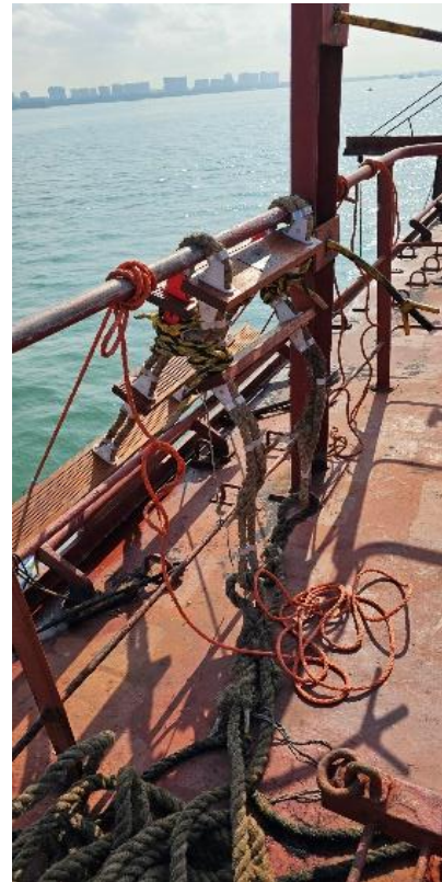
Figure 3. The pilot ladder secured to railings which is non-compliant, amongst others.
