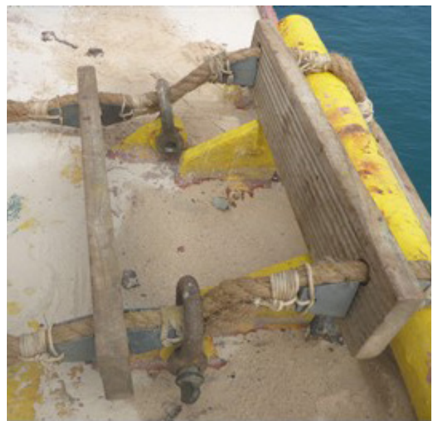
Figure 2. Pilot ladder incorrectly secured to the deck using D-shackles to choke the side ropes.
