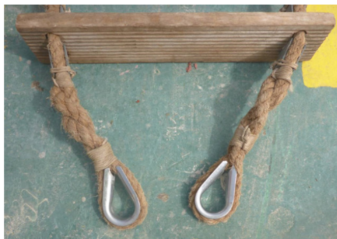
Figure 4. Pilot ladders are required to be provided at the rope ends with strong thimbles for securing the ladder.
