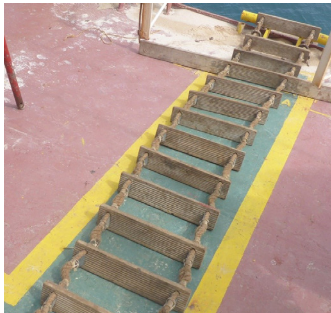
Figure 3. This ladder is too long for the freeboard.
